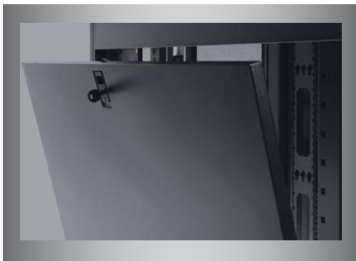
Install solid side panels to prevent hot air from recirculating around the sides of the rack enclosure.
